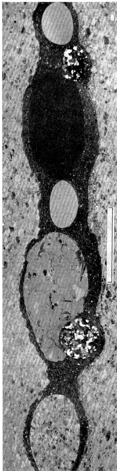
FIGURE 4. An artificially deformed conglomerate: pebbles are (from left to right) Carrara marble; oolitic limestone and quartzite; Solenhofen limestone; shale; quartzite; and Solenhofen limestone. The pebbles are set in a matrix of mica schist and plaster of paris with an outer matrix of marble. (From Gay & Jaeger 1975.)
